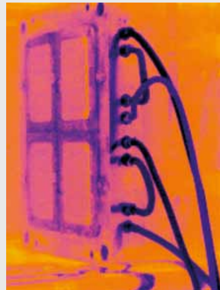
Homogenous temperature distribution in the injection mould after the temperature conditioning circuits have been cleaned.
