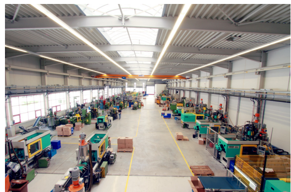
Large Windows and domes provide a high proportion of daylight in the new production hall at Goletz
